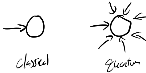
Figure 29.2: Low-energy hard sphere scattering in the classical (where the direction of scattering is limited, so \sigma = \pi a^2 ) and quantum (where the particle can scatter off of any part of the sphere, yielding \sigma = 4\pi a^2 ) cases.
